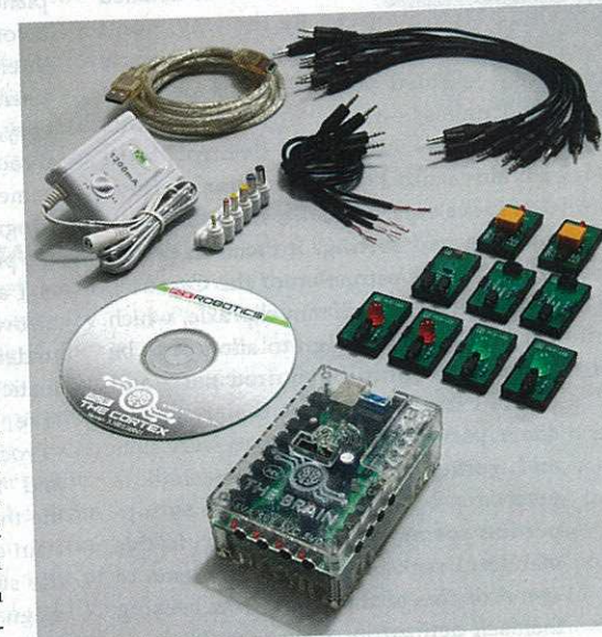
PCS Brain components (left) and fischertechnik kit parts.
