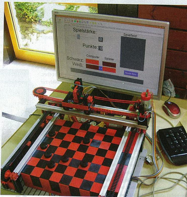
Jan Käberichs' checkers-playing ("Mühle") robot is programmed in RoboPro.
