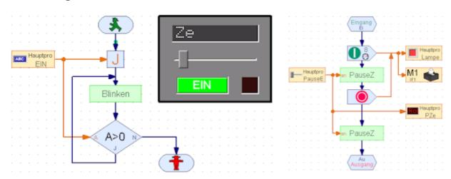
Panel elements combined for display a value and control a simple blinker. They are situated on a grey form (menu painting). The square therefore must be place in background (menu painting | object to background). The panel element are placed for a better view in the function area of the main. There is a special tab for panel elements too.
