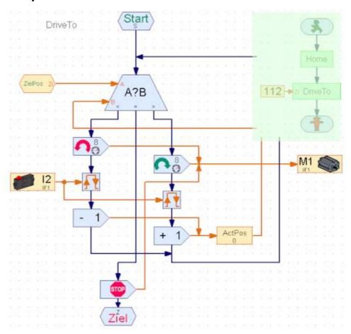
The position is noted by the parameter ZielPos (DestinationPosition). The actual position is stored in the global variable ActPos. ActPos must not to be seen in the main, but in Home. The most interesting command is A?B which compares ZielPos with ActPos. If equal, destination position is reached, motor off, return.
