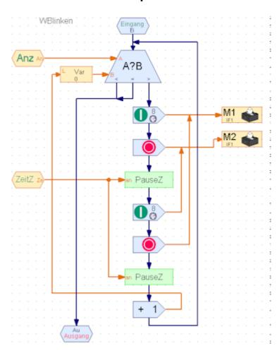
WechselBlinker has become an additional parameter Anz for the number of blinking loops (instead a fix 10). The command A?B compares parameter Anz with the actual value of the local Var (loop counter). Var is set to 0, if entering the sub. A?B has three exit pins. Two of them are connected to leave the sub on Anz<=Var.
