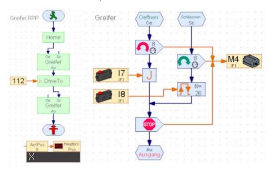
The grip differs from the other components in its operating, it is only opened and closed. But the angle to be closed is given with number of impulses. If transporting every time the same 'yellow barrell', a fix value can be choosen, may be 26.
