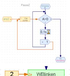
PauseZ (variable time delay) operates with a variable number of loops. The number of loops is given by a parameter stored in a local variable. Before executing the delay it is compared to 0. After the delay the local variable (Var) is decremented by 1.
