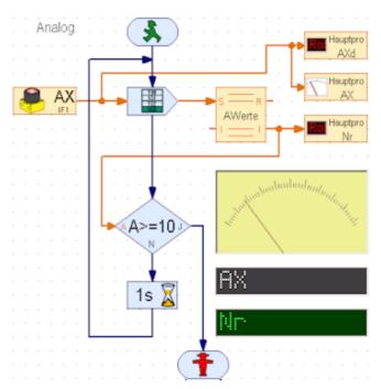
Analog scans in second intervals the actual value of the AX-Input with is connected to a photo resistor. It is displayed on the analog control and digital too. The actual list size is displayed also.
