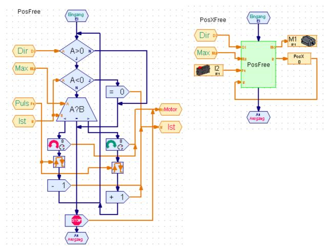
PosFree is the general sub for free movement in direction of an max position, their construction is similar to the library sub Pos (for details look their). It runs as long the button (parameter Dir A>0) ist pressed or the minimax value becomes true.
