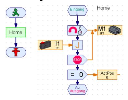
The function 'Drive to Home' now is placed in a sub using level 3 commands. A global variable ActPos is added. With larger programs the program gets more clear. Alternatively your can use the library routine PosX.
