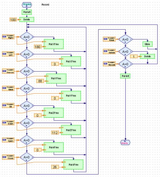
Starts with the move to home position (PosInit) and clearing the position lists (Delete, one list can contain at max 100 elements). The remaining part is dominated by a large loop in which the TeachIn buttons are scanned and the appropriate subs are called. The subs Pos\_Free have as parameter the calling button and the max-position. The max-position determine the direction of movement to, the calls therefore are always pairwise.
