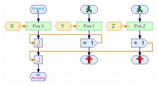
Moving to positions for the X-, Y- and Z-axis is done simultaneous in three different prozesses: The main prozess and two new one, created and – later on detroyed – while the sub is running. Each process (thread) executes one sub for postioning a robot component. The main process – after doing ist positioning work – is waiting for the two other processes to get ready. This is done with an wait for J command.
