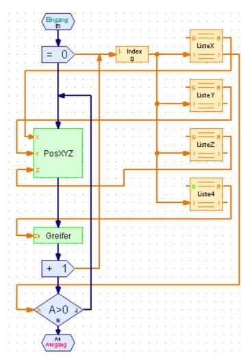
Each robot component has its own list which contain the positions to be moved to. A unchanged position never the less must be a list element.
