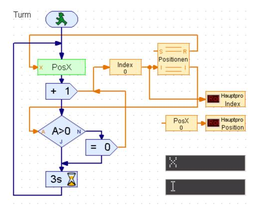
Turm moves the pile of an Industry Robots (Rob 2, 3, 4) or Computing Starter (Welding Robot) in an endless loop beginning with position 0 to 3. Therefore the list Positionen is filled with coordinate values (right click, table : 0, 45, 150, 30). The movement of the pile is done with the library routines PosX / Pos.
