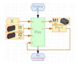
Work is done in Pos, PosX only organizes the actual parameters for the special case X-axis. The parameter X for destination position is passed through from outside.
