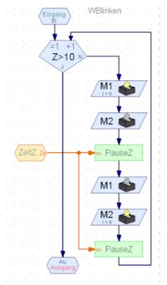
If blinking is not the only purpose of a program, to place blinking, loop included, in a subroutine.
