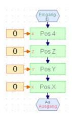
The home position of the complete robot is reached step by step with a call sub for each component. In this manner there is a good change to operate under narrow circumstances.
